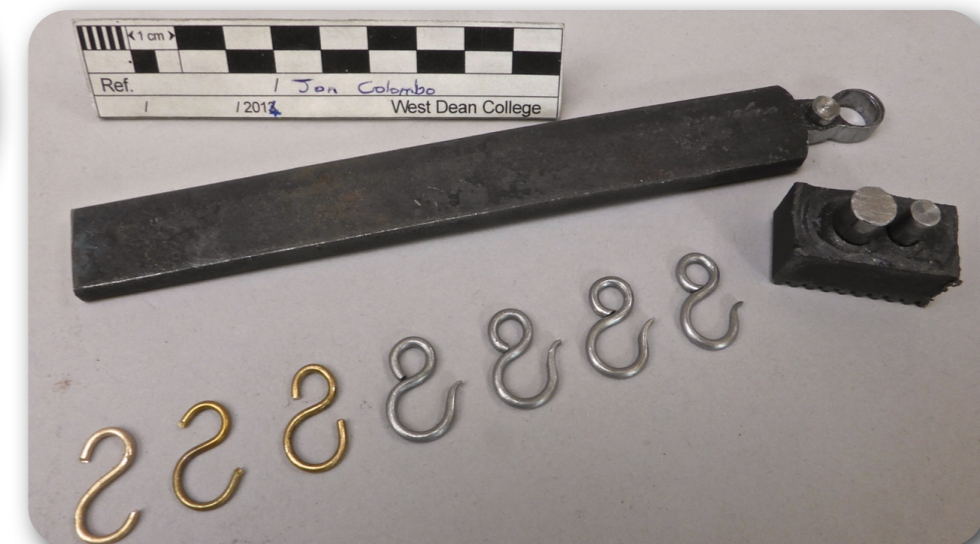
Prototype showing shrinkage patterns as found in 18th century examples
