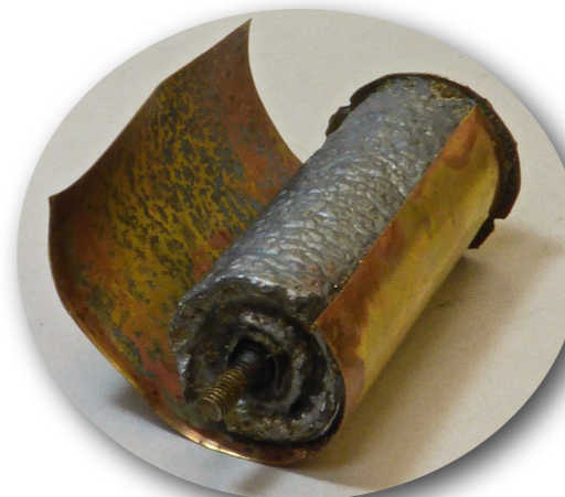
Prototype showing shrinkage patterns as found in 18th century examples
