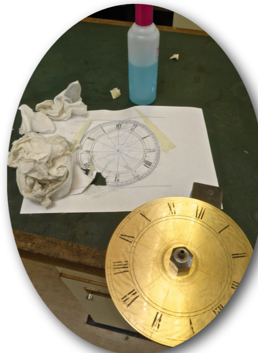
Laser transfer of the design using nail polish remover
